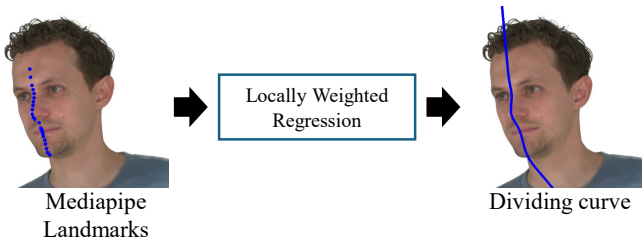
Fig. 3. An illustration of estimating the dividing curve that splits the face into two halves from Mediapipe landmarks using locally weighted regression.
